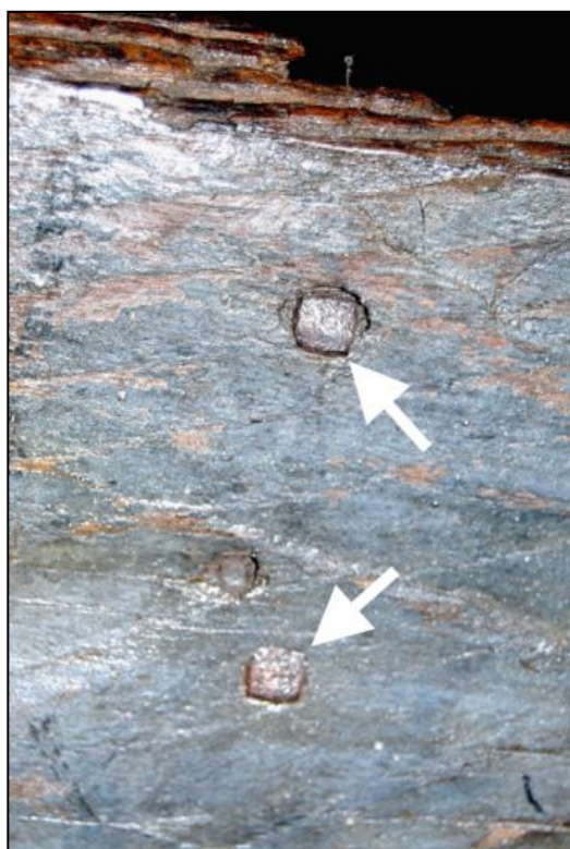
Figure 2: Detail View of Cut Nails in Gunwale
