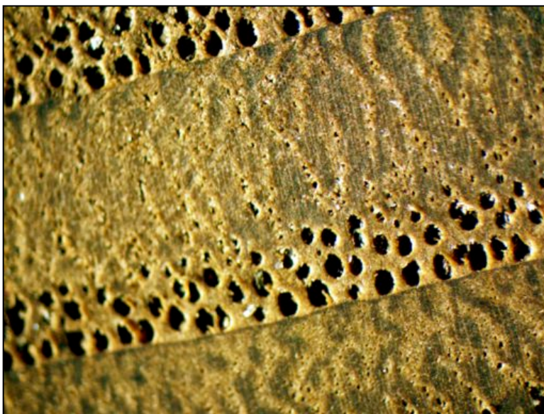
Figure 8: Transverse Section of Canoe Showing Typical Structure of Chestnut (21x)
